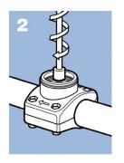
Cut hole in rigid PVC pipe using a power drill and the enclosed hole saw.
